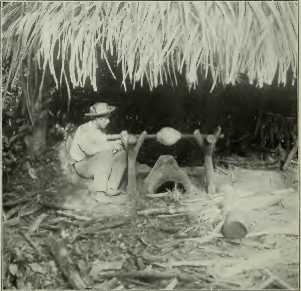
A RUBBER GATHERER SMOKING THE PRODUCT INTO A RUBBER HAM.
